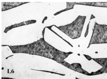
Fig. 6 Characteristic microphotograph for sample L6 (magnification \times 120 ) (light phase – primary solidified GaSb crystals; dark phase – binary eutectics (GaSb–Sn))
